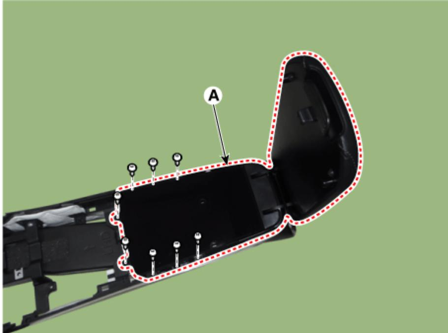
4. Disconnect the console lower side extension wiring mounting clip (A).
